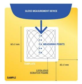
Figure 1: Schematic representation of the measuring points on the sample
